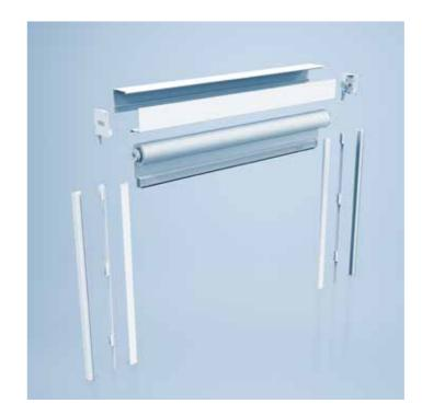
The heroal textile assembly kit supplements the components of the heroal aluminium kit with the textile assembly and the guide rail insert, which is pre-cut to size. The textile assembly includes a prefabricated fabric from the current heroal collection, a cutto-size textile roller shaft, a pre-installed motor of your choice from the heroal range, a pre-assembled end slat with weights (type III) and all other required accessories, such as roller caps and motor mounts.
